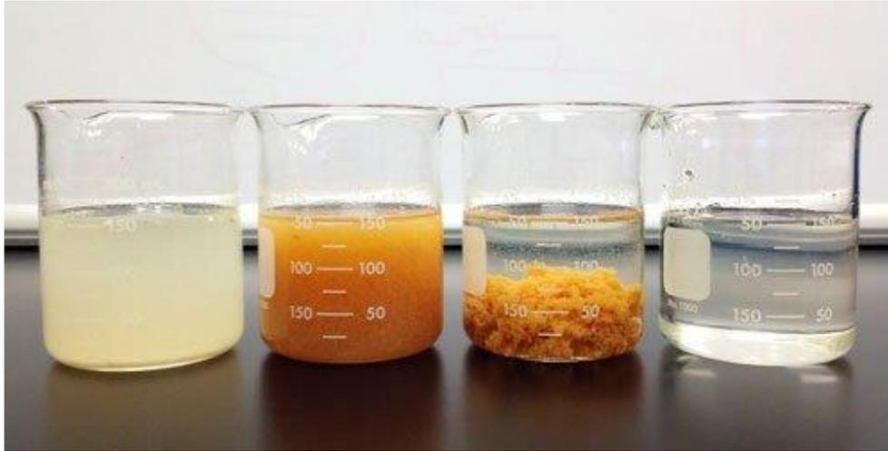
Slika 2-7 Koagulacija/flokulacija (Ecologix environmental system, 2018 )
