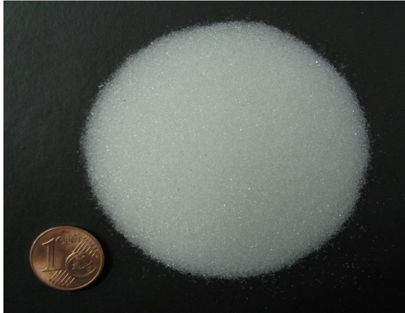
Slika 3-3 Staklene mikrokuglice (Wikipedia, 2009)
