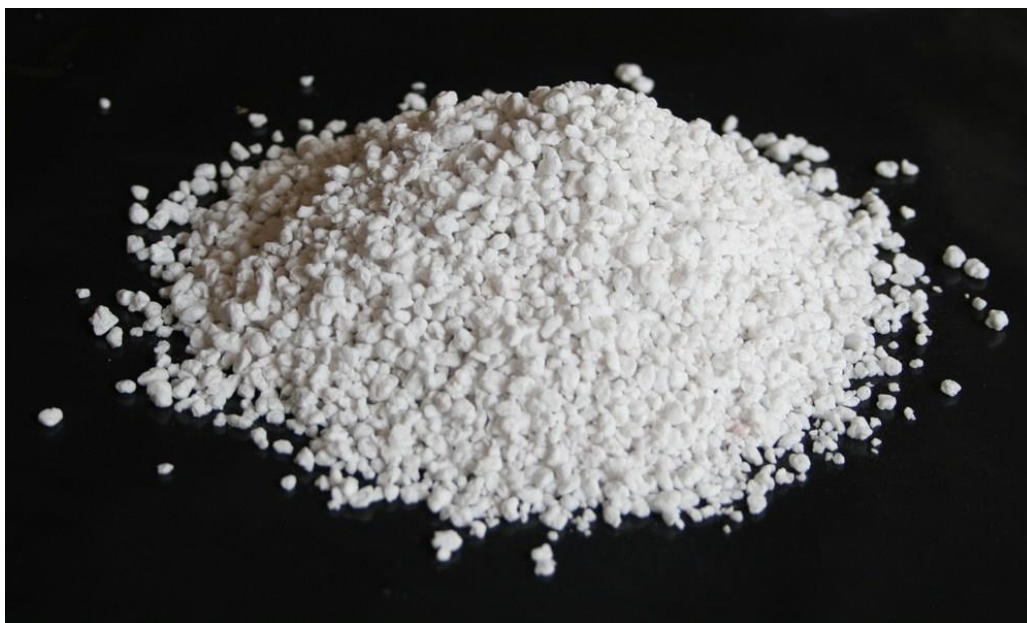
Slika 3-1 Zrnca perlita (Seedsnpots, 2018)
