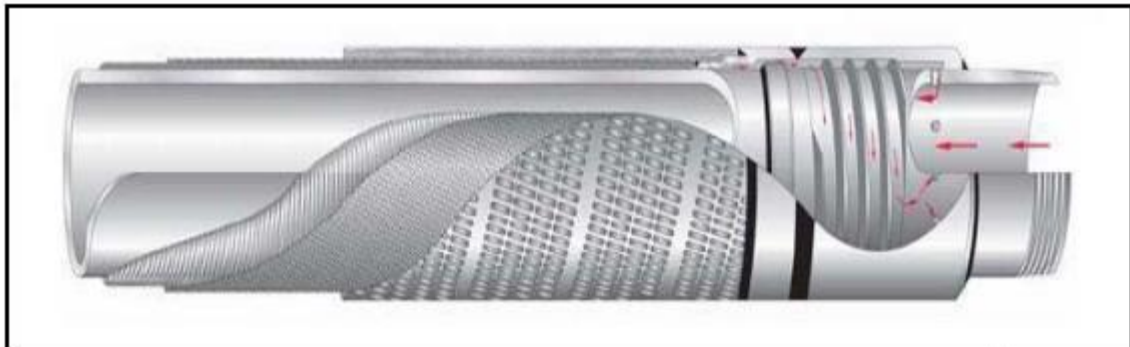
Figure 2-8. ICD helical-channel type (Al-Khelaiwi and Davies, 2007)
